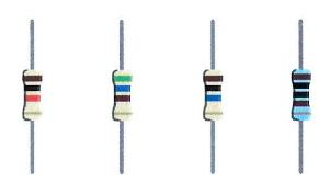
Resistors - Resist the flow of electrical energy in a circuit, changing the voltage and current as a result. Resistor values are measured in ohms (represented by the Greek omega character:  $\Omega$ ). The colored stripes on the sides of resistors indicate their value (see resistor color code table, p. 41).
