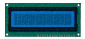
Liquid Crystal Display (LCD) - A type of alphanumeric or graphic display based on liquid crystals. LCDs are available in a many sizes, shapes, and styles. Yours has 2 rows with 16 characters each.
