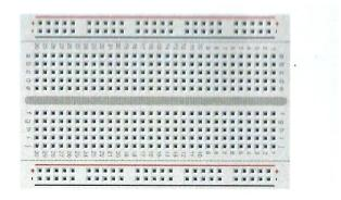
Breadboard - A board on which you can build electronic circuits. It's like a patch panel, with rows of holes that allow you to connect wires and components together. Versions that require soldering are available, as well as the solder-less type used here.
