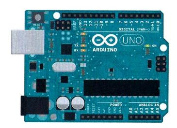
Arduino Uno - The microcontroller development board that will be at the heart of your projects. It's a simple computer, but one that has no way for you to interact with it yet. You will be building the circuits and interfaces for interaction, and telling the microcontroller how to interface with other components.
