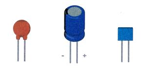
Capacitors - These components store and release electrical energy in a circuit. When the circuit's voltage is higher than what is stored in the capacitor, it allows current to flow in, giving the capacitor a charge. When the circuit's voltage is lower, the stored charge is released. Often placed across power and ground close to a sensor or motor to help smooth fluctuations in voltage.
