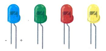
Light Emitting Diodes (LEDs) - A type of diode that illuminates when electricity passes through it. Like all diodes, electricity only flows in one direction through these components. You're probably familiar with these as indicators on a variety of electronic devices. The anode, which typically connects to power, is usually the longer leg, and the cathode is the shorter leg.
