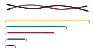
Jumper wires - Use these to connect components to each other on the breadboard, and to the Arduino.
